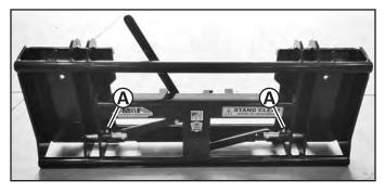
1. Lubricate the two grease fittings (A) until grease appears in the joints.
