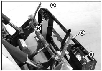
3. Move the loader attaching plate levers (A) to the unlocked (up) position either manually or by using the loader controls.
