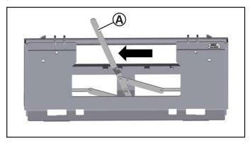
3. Move the Adapter lever (A) to the unlocked position.
