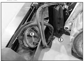
• If the attachment is assembled for operation with the boom sideways, route the hoses through the two guides (E) as shown.
