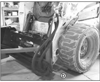
• If the attachment is assembled for operation with the boom out, route the hoses through the guide (D) as shown.
