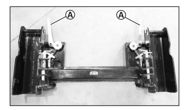
1. Move the wedge levers (A) to the upright position as shown before installing on the tractor loader.
