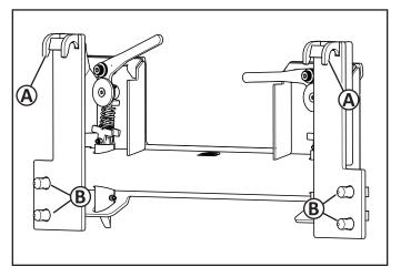
2. Follow the instructions to remove the loader holder and holder strap from the Adapter hook (A) and pin (B).
