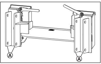
2. Follow the instructions to remove the loader pins from the holes in the mounting brackets (A).
