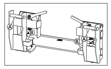
2. Follow the instructions to remove the loader carriers and pins from the Adapter pins (A) and brackets (B).
