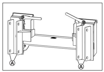
2. Follow the instructions to attach the loader pins to the holes in the mounting brackets (A).
