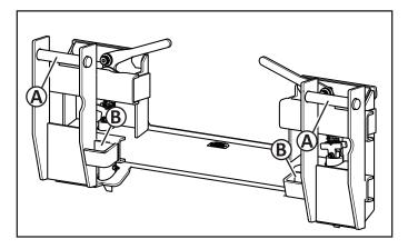
2. Follow the instructions to attach the loader carriers and pins to the Adapter pins (A) and brackets (B).
