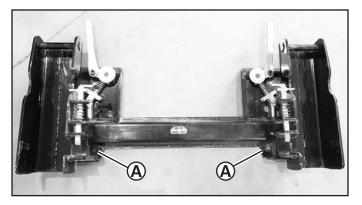
1. Lubricate the two grease fittings (A) until grease appears in the joints.
