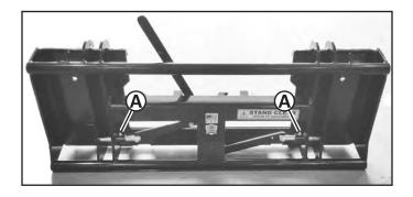
1. Lubricate the two grease fittings (A) until grease appears in the joints.
