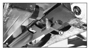
Picture Note: Adapter wedge pin on left side of skid steer attachment shown. Check the wedge pins on both sides of the attachment.
