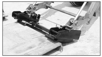
Picture Note: For easier installation on some loader models you may need to tilt the Adapter at an angle as shown.
