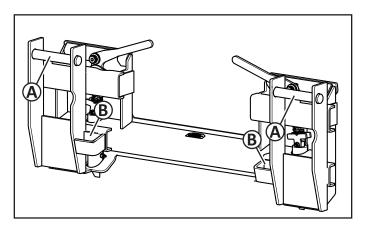
2. Follow the instructions to remove the loader carriers and pins from the Adapter pins (A) and brackets (B).
