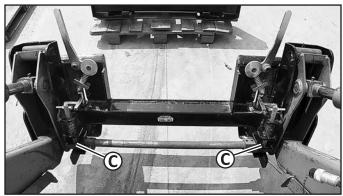
5. Check to be sure the pins (C) have dropped to secure the Adapter to the tractor loader.
