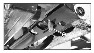
Picture Note: Adapter wedge pin on left side of skid steer attachment shown. Check the wedge pins on both sides of the attachment.
