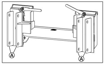
2. Follow the instructions to remove the loader pins from the holes in the mounting brackets (A).
