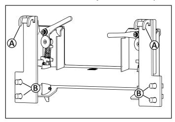
2. Follow the instructions to attach the loader holder and holder strap to the Adapter hook (A) and pin (B).
