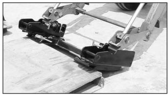
Picture Note: For easier installation on some loader models you may need to tilt the Adapter at an angle as shown.
