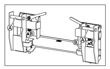
2. Follow the instructions to attach the loader carriers and pins to the Adapter pins (A) and brackets (B).
