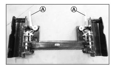
1. Move the wedge levers (A) to the upright position as shown before installing on the tractor loader.
